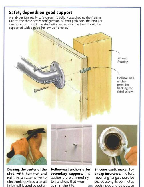
method to determine the exact position of the stud's edges and center.
